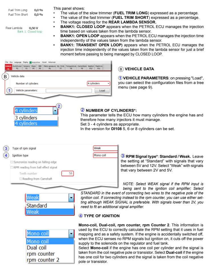
NOTE: some engines with one coil per cylinder may need this selection. In other cases, select the **rpm counter** option. Select **rpm counter** 2 if the rpm levels seen in the "rpm counter" setting are two times the real value.
