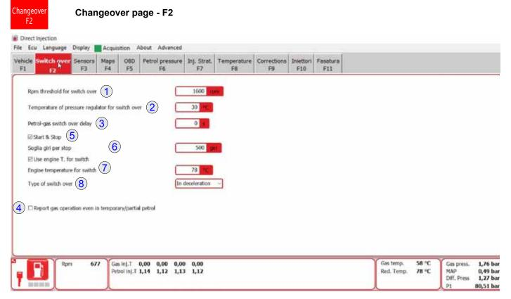
**(1) RPM THRESHOLD FOR CHANGEOVER** (range 0-3000 RPM): identifies the RPM at which the switch over from PETROL TO GASoccurs.
