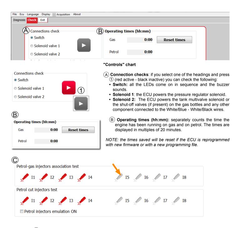
(C) **Petrol-gas injector association test:** this lets you test that the gas injectors are working properly and that they are correctly associated with the petrol injectors. Click on the gas injector you want to test (while running on gas), the symbol will change colour and the corresponding cylinder will be fuelled with petrol. This function allows you to carry out various checks:
