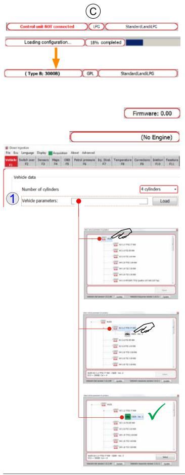
**LPG - CNG** - shows the type of fuel selected when the program is being saved (the type of fuel can be selected from the sub-menu "Type of fuel " on the "Vehicle - F1") page.
