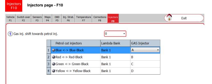
Phasing can be set between the injector on which petrol injection is detected and the injector through which gas is injected. This parameter is known as "Gas injector phasing in relation to petrol".
